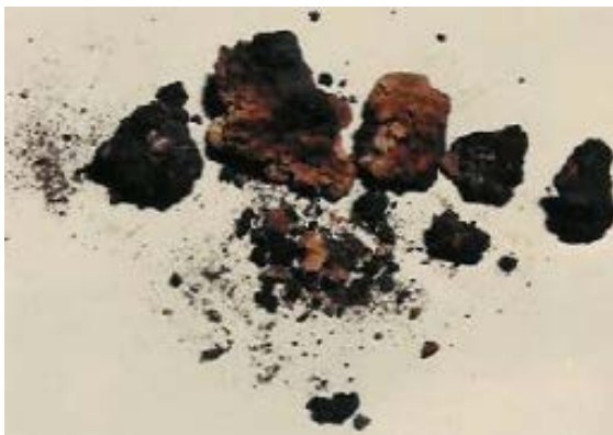
Figure 9: Charred product from the engine compartment of a wheel loader (Figure: Prof. Siegfried Radandt)
