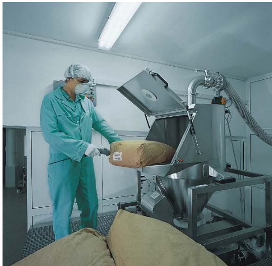
Figure 1: Bag emptying station with connection to a central exhaust system (Figure: AZO GmbH + Co. KG)
