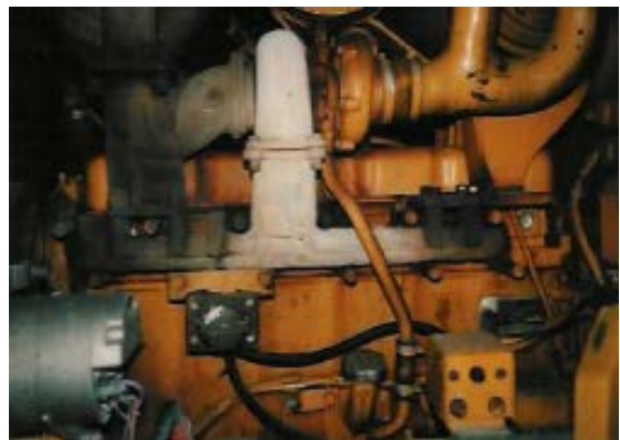
Figure 9: Charred product from the engine compartment of a wheel loader (Figure: Prof. Siegfried Radandt)
