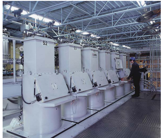
Figure 2: Bag emptying stations with integrated filters (Figure: AZO GmbH + Co. KG)
