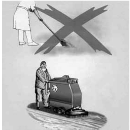
Figure 3: Improper and proper methods for removing flammable dust
