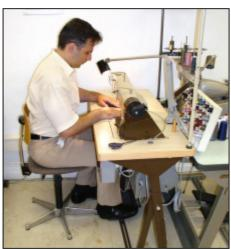
Swivel chairs for workstations are approved in accordance with the DIN 68877 standard. These chairs are adjustable in height, seat tilt, and backrest position and their backrest is padded. They facilitate the necessary work and support the worker's spine.
