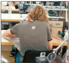
If the height of the table, including the sewing machine, is too low, the worker must hunch forward in order to properly view the sewing needle. In such a position it is difficult to operate the treadle.
