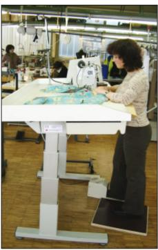
A frame which allows you to adjust the height of the sewing machine fulfills the requirements for an optimal sewing workstation and also allows you to change between sitting and standing thereby reducing one-sided and mainly static posture.
