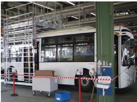
Figure 8: Example of safeguarding of the working area during testing work
