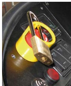
Figure 2: Examples of safeguarding against reconnection
