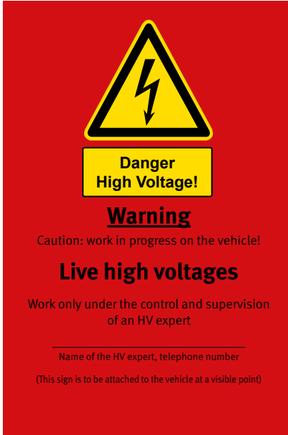
Figure 6: Marking of HV vehicles in the workshop
