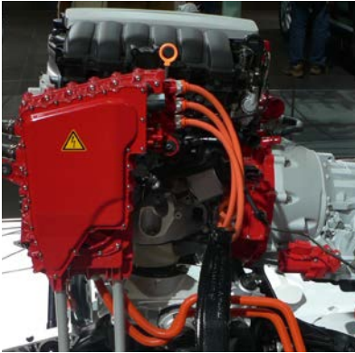
Figure 5: Basic protection by isolation and shrouding
