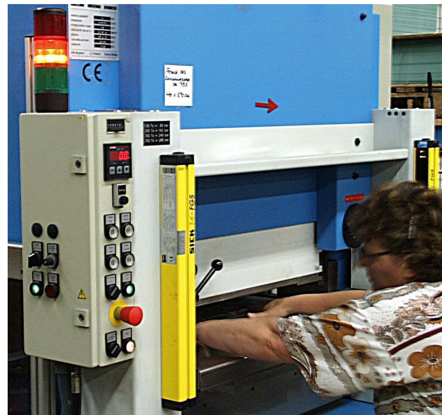
Protection of a punching machine by a light curtain
